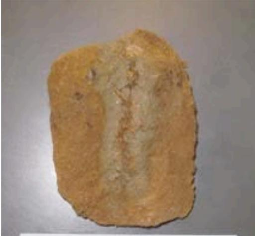
Figure 2. Sample 1d, showing the reddish matrix surrounding a vertically elongated gray zone that is centered along a crack filled with red clay.
