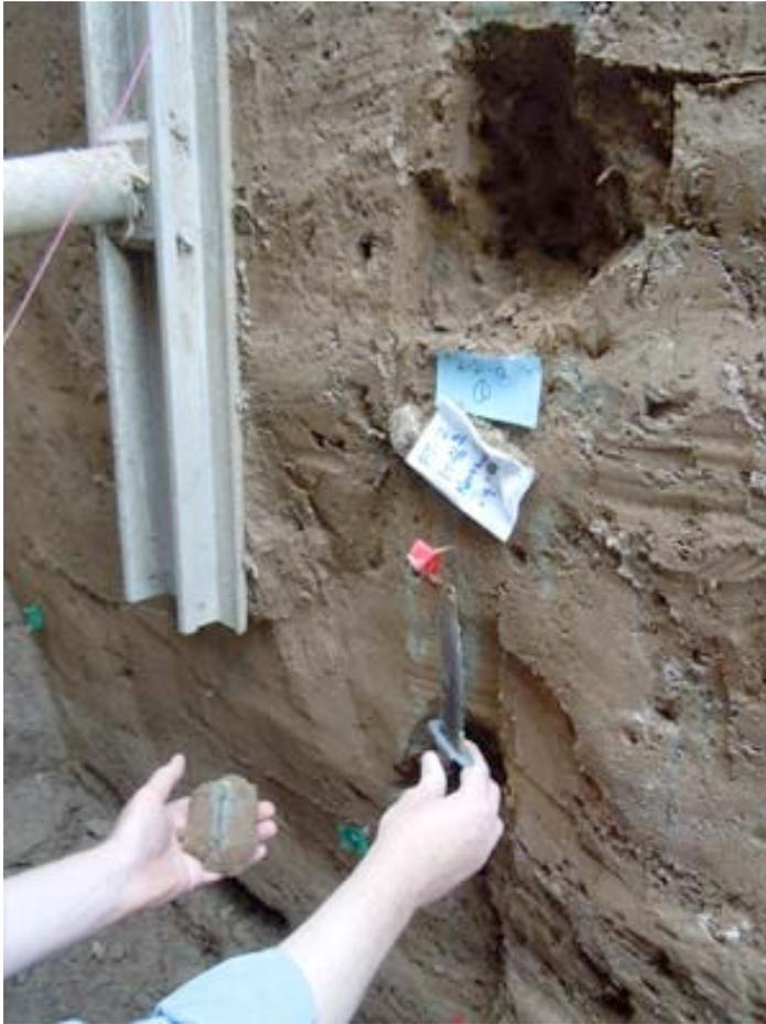
Figure 1. *Sample Site 1: FT-2, 1+46.5, North wall - 9'*. Samples 1a, b, c were taken above the blue card, Sample 1d is held in hand and was taken below the red tape. Note blue zones within the general reddish soil matrix.
