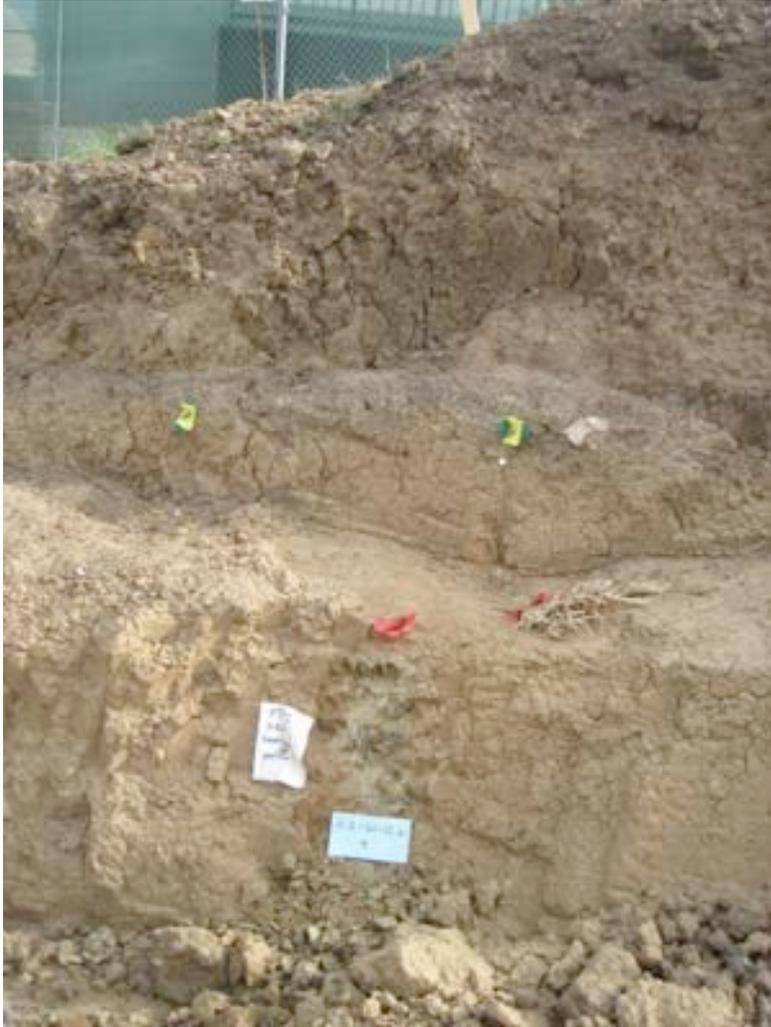
Figure 11. *Sample Site 4: FT-2, 1+50, South wall near surface. Sample was taken from the gray zone above the blue card.*
