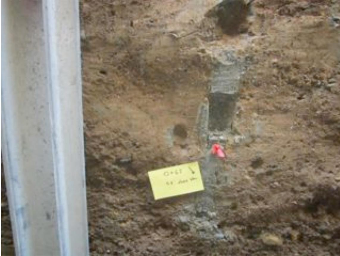
Figure 8. Sample Sites 9 & 10: FT-5, 0+62, West wall, 4.8' above bottom of trench. Sample 9 is from gray material. Gray material extends back only about 10 cm into the trench wall. The feature may be a krotovina (back-filled rodent burrow). Sample 10 is 20 cm to left of Sample 9.
