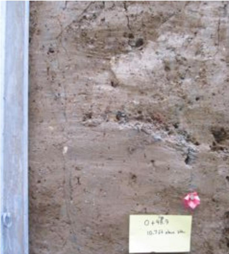
Figure 6. Sample Sites 7 & 8: FT-5, 0+48.9, West wall, 10.7' above bottom of trench. Gray seams around cracks within 1 m of the surface. Sample 8 is 30 cm above Sample 7.
