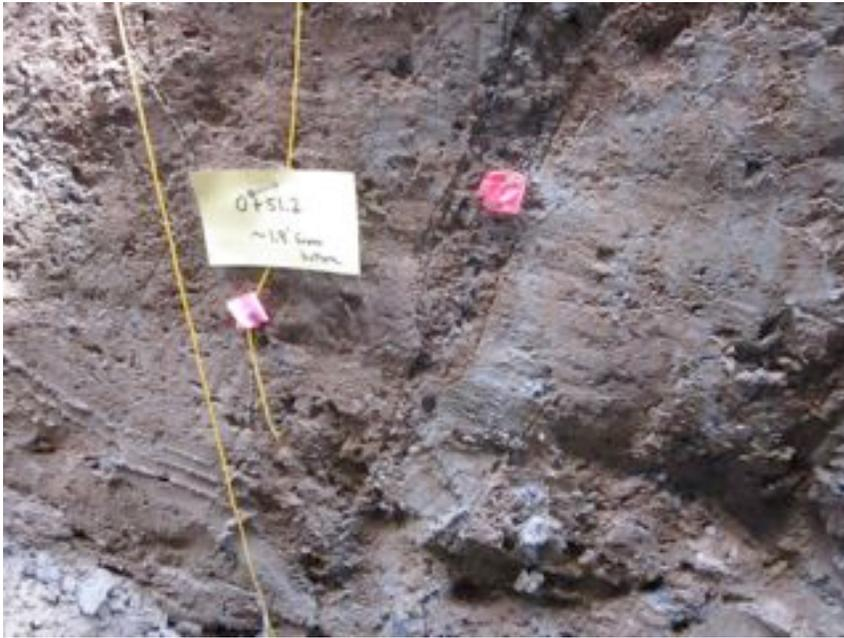
Figure 1. Sample Sites 1 – 3: FT-5, 1+51.2, East wall, 1.8' from bottom. Sample 1 -- infilled coarse material in fault; Sample 2 -- just below Sample 1; Sample 3 -- gray material to right of fill/fault.
